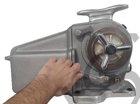
Remove the stripper by unscrewing the two M8 screws.
